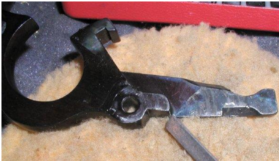
See the cam After the sharp edge was removed.
